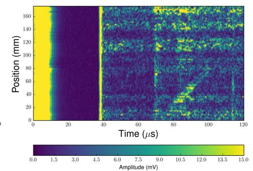
Figure 7: B scan image from a cast sample cut from a severely cracked slab.
