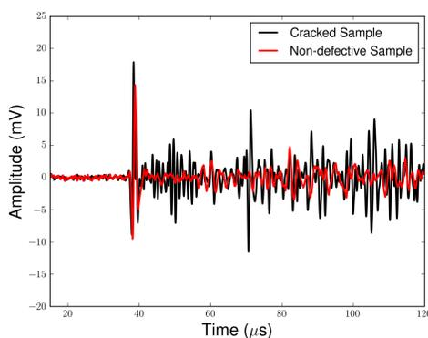
Figure 8: A comparison of amplitude data from the non defective sample from fig. 6. and from a defective region of fig. 7.
