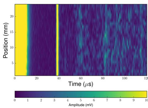
Figure 6: B scan image from a non-defective cast sample.
