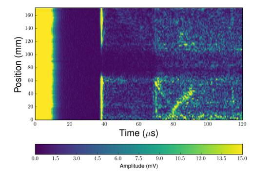
Figure 9: B scan image from a cast sample with a visible crack through the full cast thickness.
