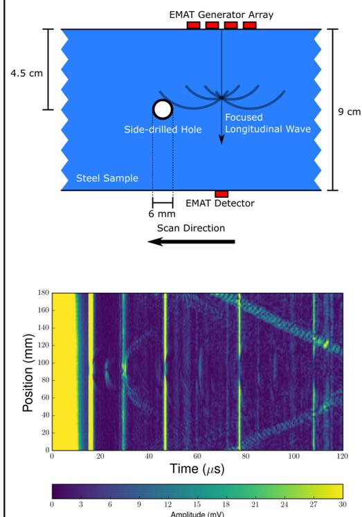
Figure 4: B scan image of the test block showing a defect indication at 90 mm.
