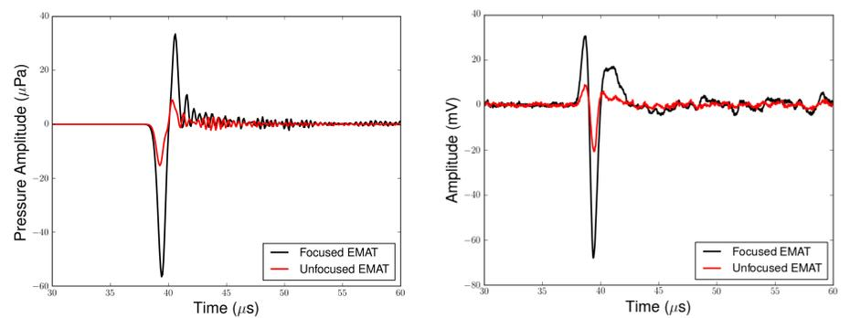
Figure 2: Simulated (left) and experimental (right) data demonstrating signal enhancement from phased array generation using EMATs.
