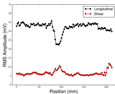
Figure 5: Amplitude variation of transmitted longitudinal and shear modes in the B scan.
