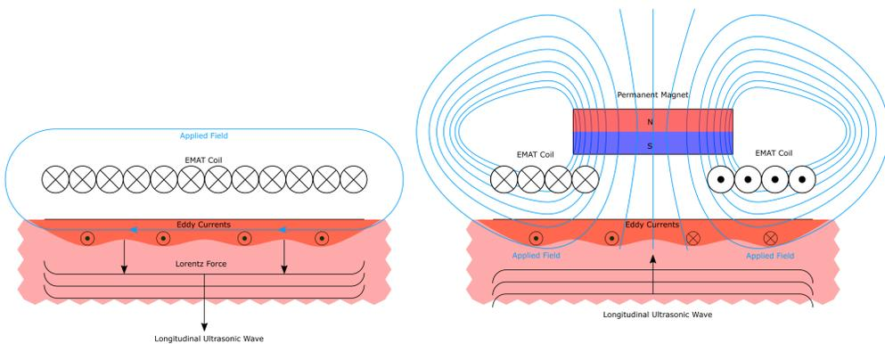
Figure 1: Schematic diagrams of a self-field EMAT generator (left) and detection EMAT (right).
